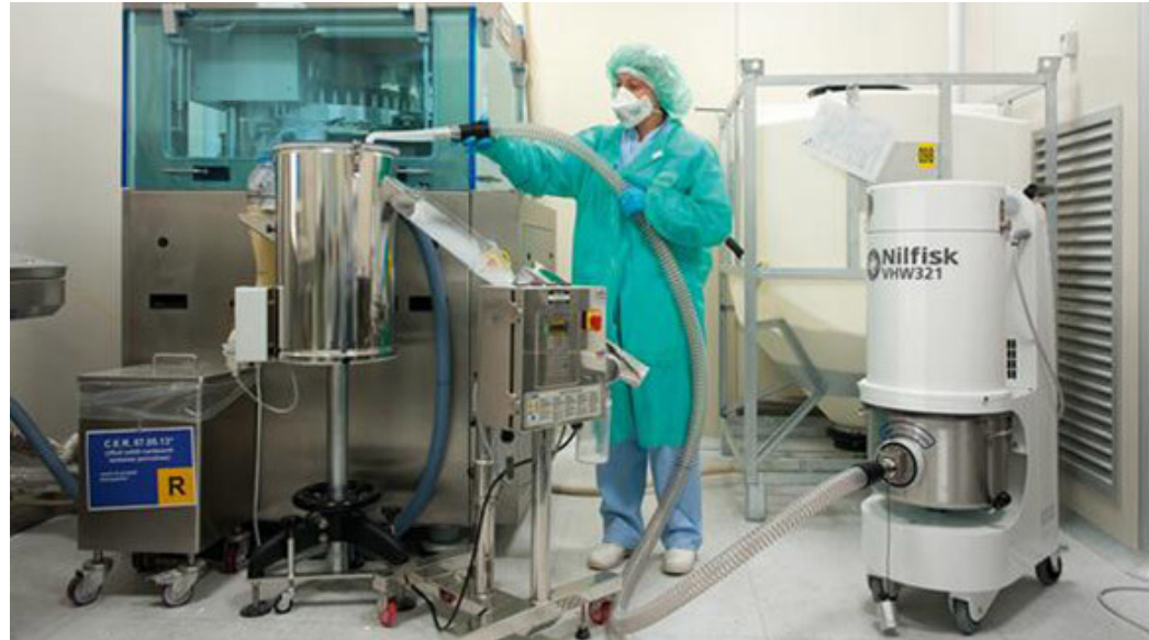
Removing residual API from filling reservoir of tablet press
