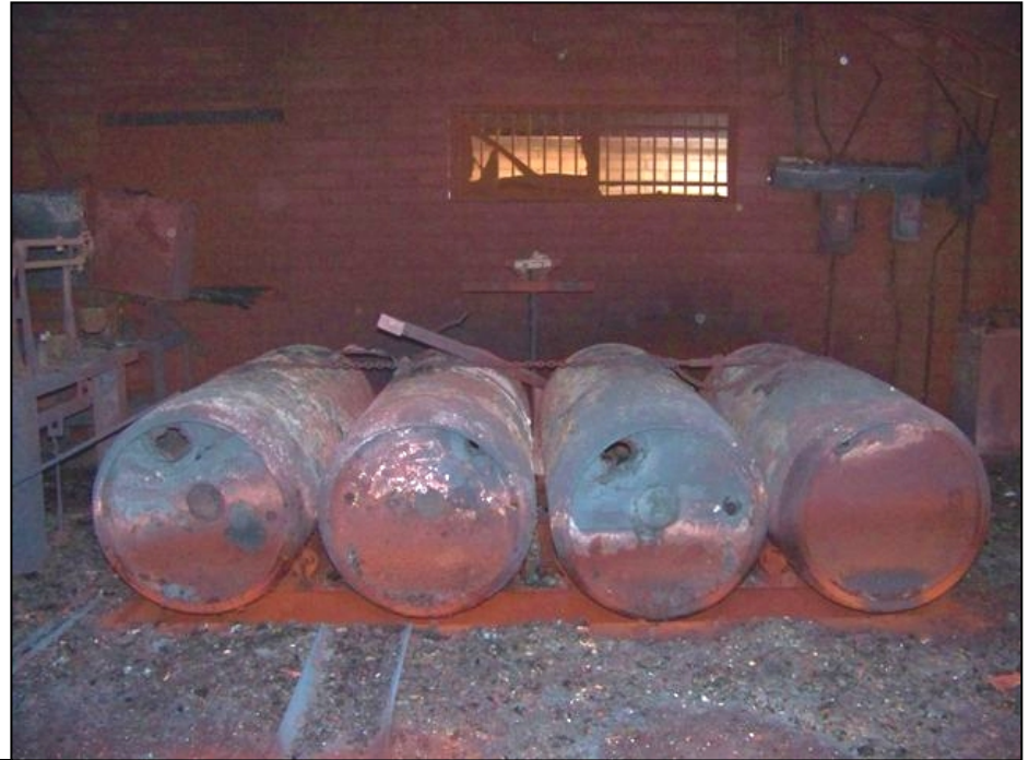
One-ton containers burned in the 2007 “Rice Fire” at the Red Mountain Chlorination Facility (photos courtesy of Mike Page, Fallbrook Public Utility District.)
