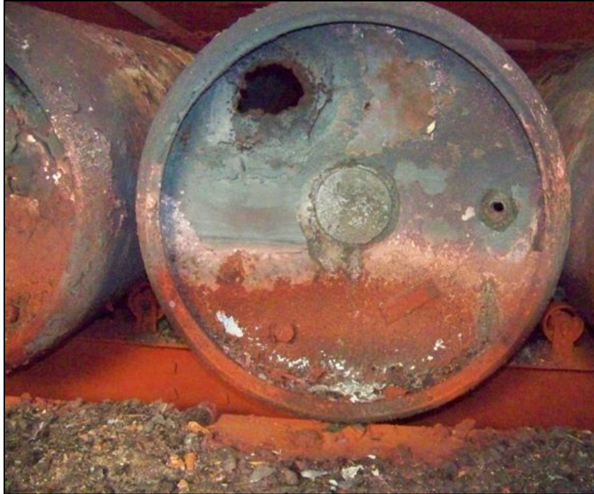
One-ton containers burned in the 2007 “Rice Fire” at the Red Mountain Chlorination Facility (photos courtesy of Mike Page, Fallbrook Public Utility District.)
